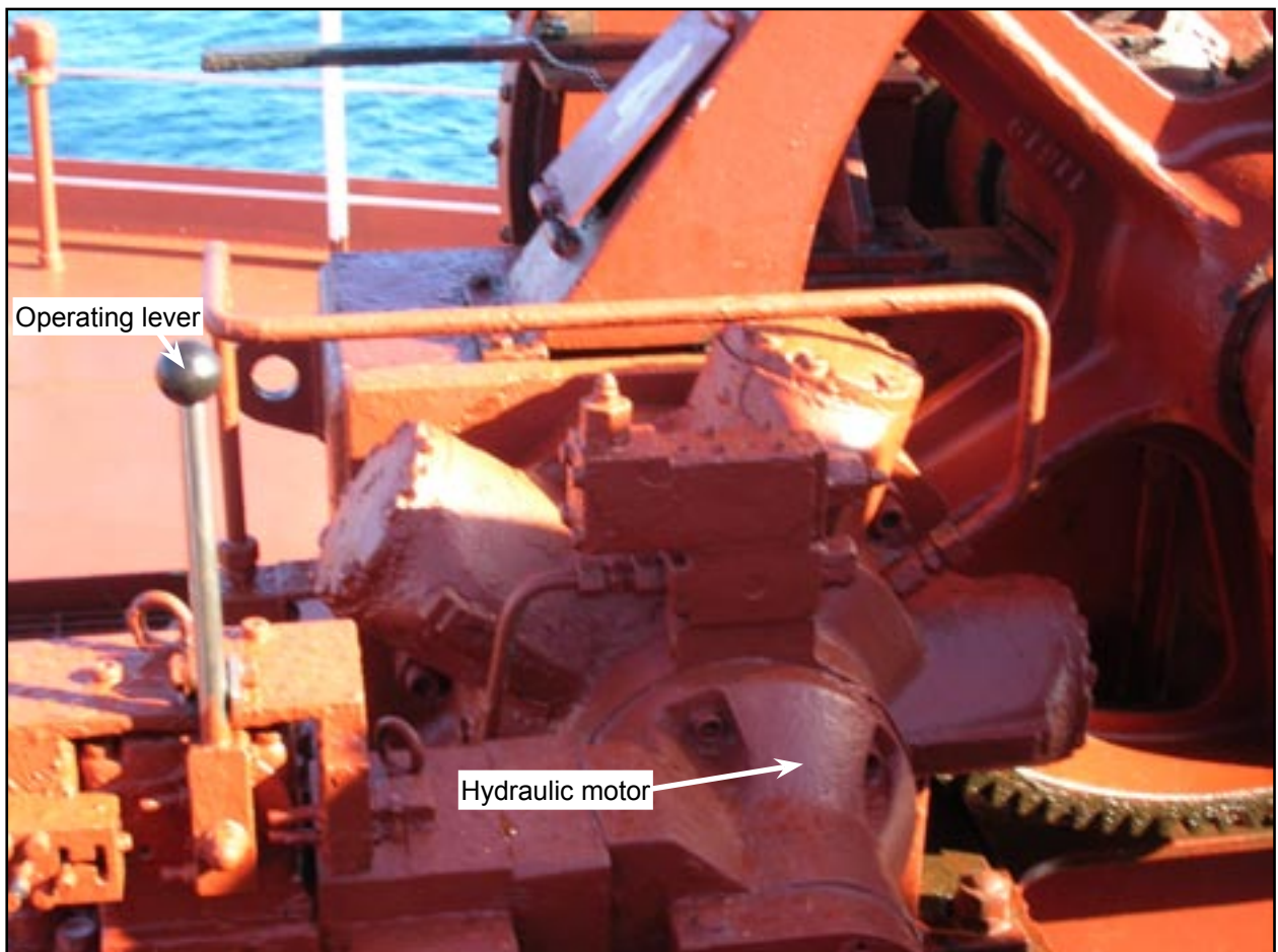
Port Windlass Hydraulic motor
