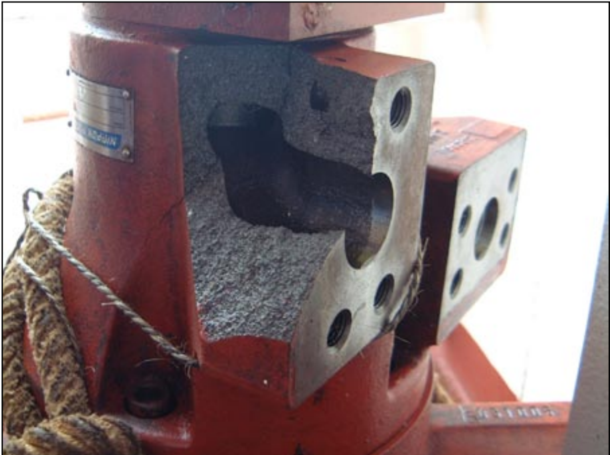
Damage to the port windlass hydraulic motor unit
